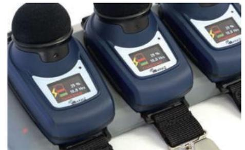
When placed in any of the three 'pockets' the dBadge2 will also begin to charge the battery displaying it's charge status in terms of % charge and projected run time (based on how the dBadge is configured). To check progress, simply press either key or tilt the docking station to 'wake' the dBadge2. A complete charge from empty will take 6 hours, whilst a charge sufficient to conduct an 8 hour survey will take just over an hour.
